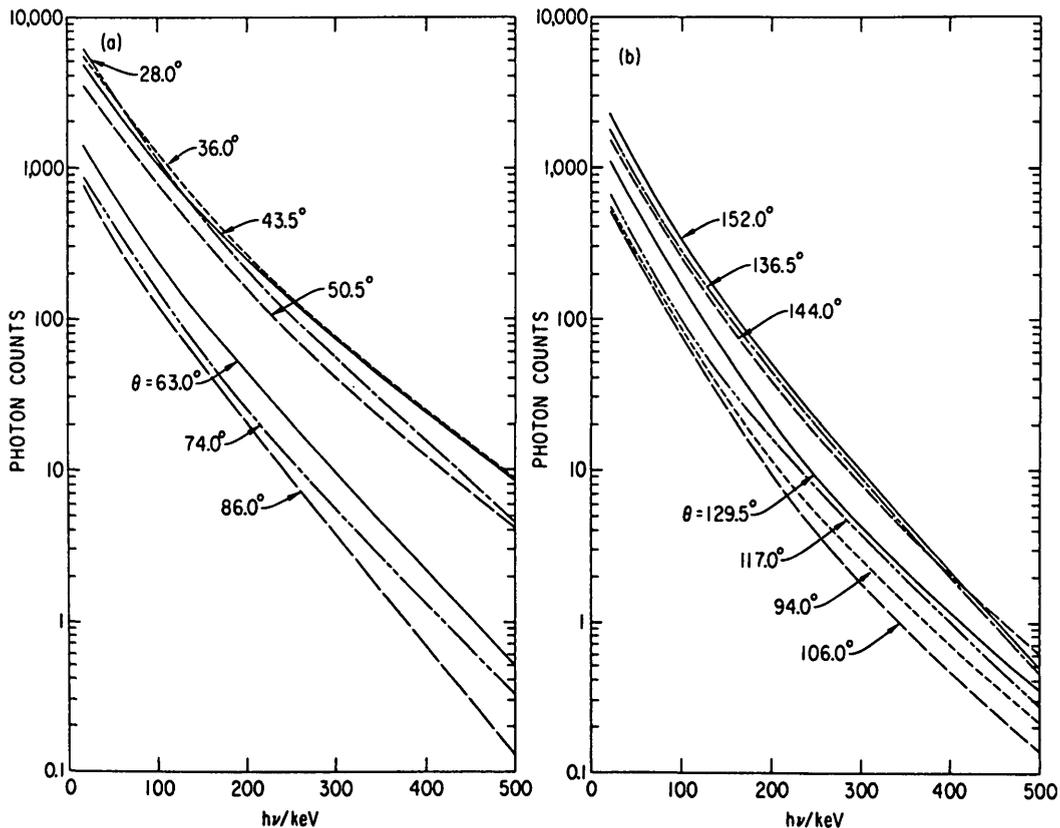
FIG.9. Fitted spectra with detector angle  $\theta$  as parameter for normal discharge (a) and for reversed discharge (b). No geometry correction has been applied yet.
