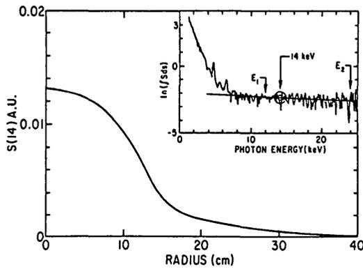
FIG. 10. Abel-inverted radial profile of X-ray intensity at  $h\nu = 14$  keV photon energy obtained with soft-X-ray PHA system. Insert shows typical soft-X-ray spectrum. Tail is fitted between energy  $E_1$  and  $E_2$  by straight line in order to obtain X-ray emission at photon energy of 14 keV.
