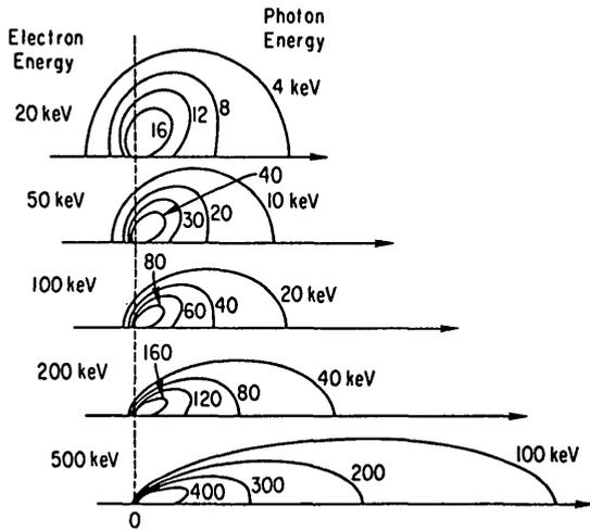
FIG.1. Bremsstrahlung emission cones for mildly relativistic electrons.
