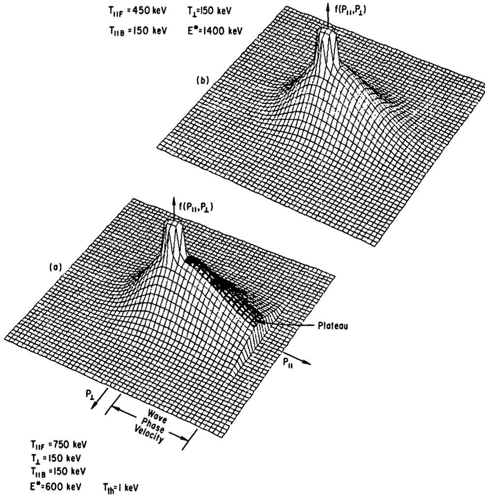
FIG.12. Two distribution functions fitting tangential scan discussed in Section 3. Plateau, thought to be created by Landau damping of lower-hybrid waves, is indicated by shading in (b). Height of distribution function is plotted on linear scale.
