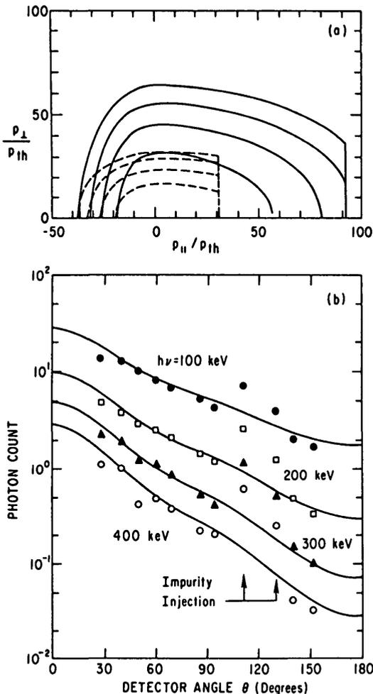
FIG.19. Tangential scan of runaway discharge. Parameters for bremsstrahlung fit of data: parallel forward temperature  $T_{\parallel F} = 1400$  keV, maximum energy  $E^* = 2500$  keV, perpendicular energy  $T_{\perp} = 450$  keV, backward temperature  $T_{\parallel B} = 140$  keV, backward fraction  $f_B = 1$ . For comparison, electron distribution during lower-hybrid current drive is indicated by dashed lines in (a). Each contour represents a factor of 10.
