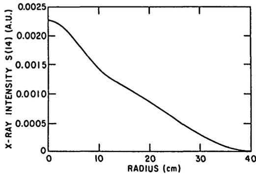
FIG.16. Radial profile of X-ray emission at photon energy of 14 keV for low-magnetic-field discharge (toroidal magnetic field  $B_T = 20$  kG, plasma current  $I_p = 270$  kA).
