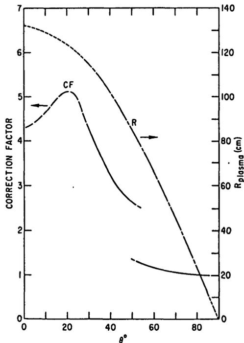
FIG. 6. Typical geometry-correction factor (CF) for tangential detector viewing plasma along chord tangential to circle with major radius  $R$  at angle  $\theta$  with respect to PLT magnetic axis. Exact shape of correction factor depends on radial emission profile. Curve presented here is based on radial profile shown in Fig. 10.
