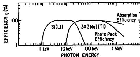
FIG.3. Photo peak and absorption efficiency for lithium-drifted silicon Si(Li) and for 3 in. X 3 in. sodium iodide NaI (Tl) detectors used for PLT experiments.
