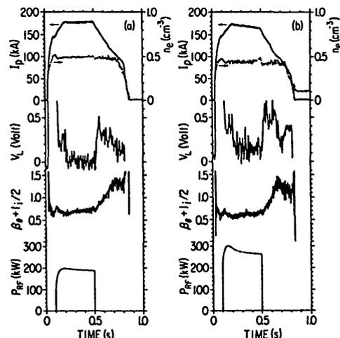
FIG. 7. Plasma conditions for lower-hybrid current-drive discharge discussed in Section 3. Plotted are plasma current  $I_p$ , line-average electron density  $\bar{n}_e$  from microwave interferometer, plasma loop voltage  $V_L$ , Shafranov parameter  $\beta_\theta + \xi_i/2$ , and RF power versus time. (a) plasma current in normal direction; (b) plasma current in reverse direction.
