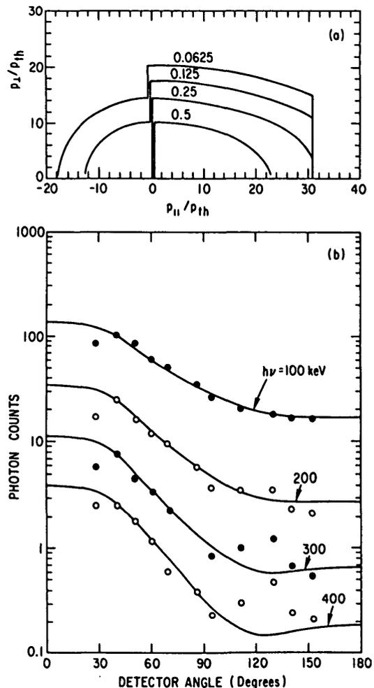
FIG.17. Tangential scan of hard-X-ray emission for low toroidal magnetic field. Parameters for fit are: forward temperature  $T_{\parallel F} = 750$  keV, perpendicular temperature  $T_{\perp} = 150$  keV, backward temperature  $T_{\parallel B} = 225$  keV, maximum electron energy  $E^* = 600$  keV, backward fraction  $f_B = 0.25$ .
