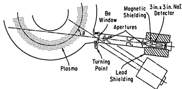
FIG.2. Schematic of tangential hard-X-ray detector on PLT.
