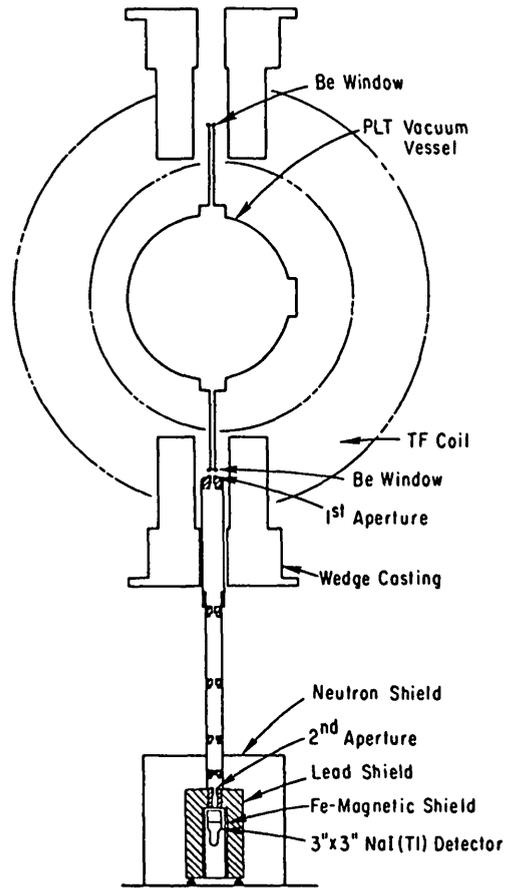
FIG.4. Schematic of vertical hard-X-ray detector on PLT.
