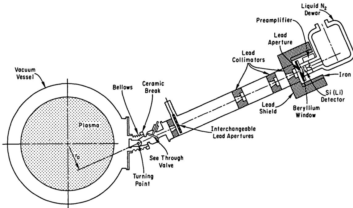
FIG.5. Schematic of soft-X-ray PHA system used to obtain radial profiles of hard-X-ray emission on PLT.
