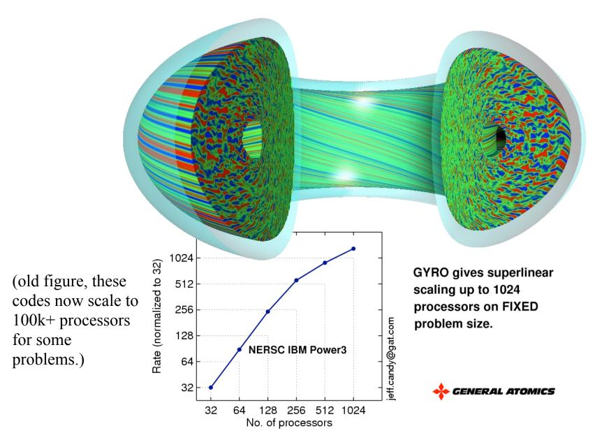
Comprehensive 5-D computer simulations of core plasma turbulence being developed by Plasma Microturbulence Project. Candy & Waltz (GA) movies shown: d3d.n16.2x\_0.6\_fly.mpg & supercyclone.mpg, from <u>http://fusion.gat.com/comp/parallel/gyro\_gallery.html</u> (also at <u>http://w3.pppl.gov/~hammett/refs/2004</u>).
