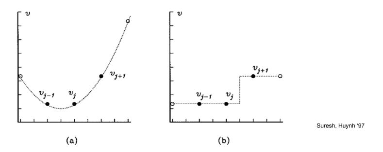
**FIG. 2.1.** An extrema and a discontinuity look the same over a stencil of three points. The values  $v_{j-1}$ ,  $v_j$  and  $v_{j+1}$  in (a) are identical to the corresponding ones in (b).
