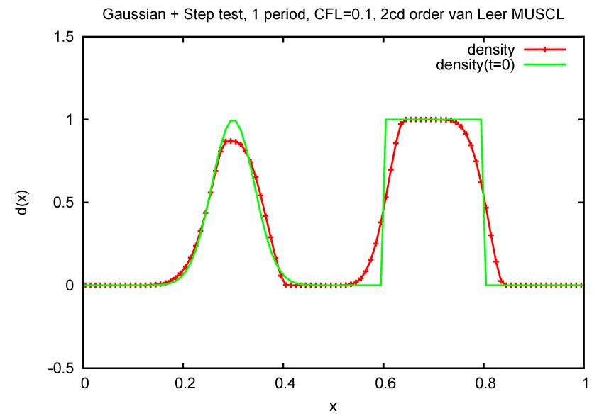
3<sup>rd</sup> order SSP-RK used here. Looks better at CFL=0.5 with 2cd order single-step time-space-coupled time advancement, (becomes exact at CFL=1), but for complex flows there will be regions at many different values of CFL=v\*dt/dx, incl. CFL<<1.
