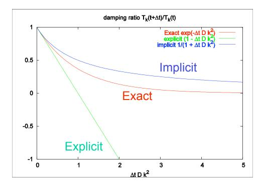
Implicit algorithm is accurate for modes with small  $\Delta t D k^2$ , while robustly stable for all  $\Delta t D k^2$ , giving qualitatively correct damping for all modes.
