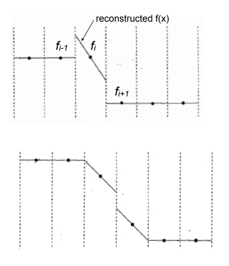
Central differencing around boundary,  $s_i = s_{i+1/2} = (f_{i+1} - f_i)/\Delta x$ , corresponds to a reconstructed f(x) that has overshoots. Even central differencing around a cell,  $s_i = (f_{i+1} - f_{i-1})/(2\Delta x)$  would give overshoots.
