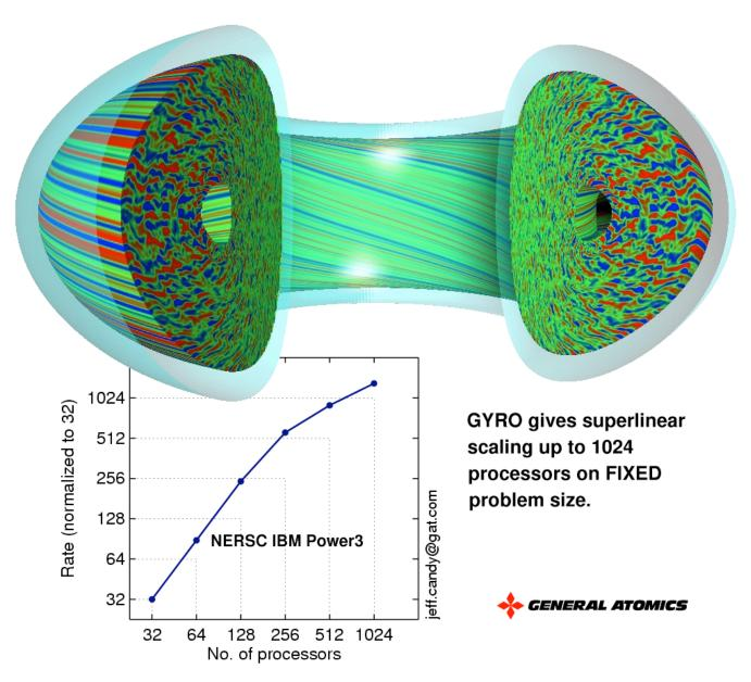
Comprehensive 5-D computer simulations of core plasma turbulence being developed by Plasma Microturbulence Project. Candy & Waltz (GA) movies shown: d3d.n16.2x\_0.6\_fly.mpg & supercyclone.mpg, from <u>http://fusion.gat.com/comp/parallel/gyro\_gallery.html</u> (also at <u>http://w3.pppl.gov/~hammett/refs/2004</u>).
