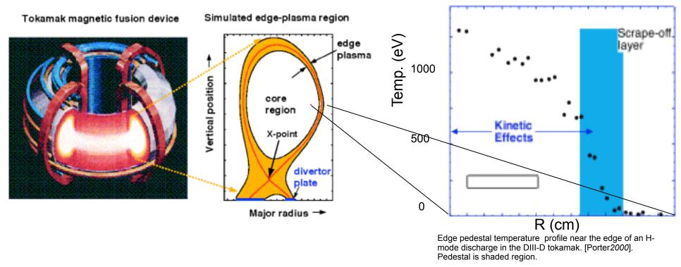
Major extensions to gyrokinetic codes needed to handle additional complications of edge region of tokamaks (& stellarators):
