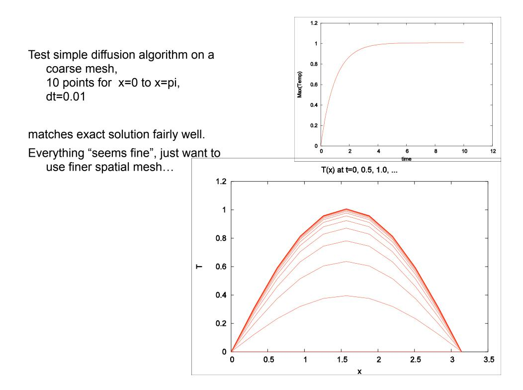
Test simple diffusion algorithm on a finer mesh, increase from 10 to 100 points for x=0 to x=pi, dt=0.01 (unchanged)
