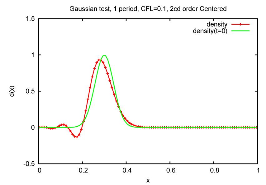
Relatively okay solution, will converge to exact solution as  $\Delta x \rightarrow 0$ . But disappointing it requires so many grid points, and that there are artificial oscillations and that f<0.
