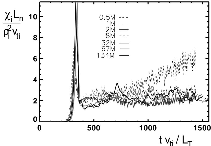
Typically need 2-4 particles per cell (1-2 M in this case), or more particles near marginal stability.
