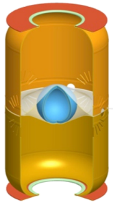
Fig. 58: Target suspended by the “tent” within the hohlraum.
