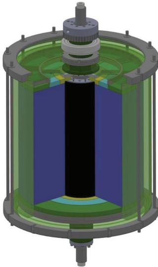
FIG. 1. (Color online) Drawing of the HTX device illustrating the segmented axial boundaries: the innermost element (yellow) is connected to the inner cylinder (black), the outermost element (green) is connected to the outer cylinder (green), and the middle components (blue) are rings that can rotate differentially with respect to the cylinders.
