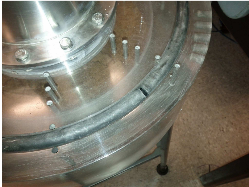
Figure 2.3: Picture of gasket used to minimize axial pressure loads on the outer ring. The gasket is the black rubber piece fitted into the groove machined near the outer diameter of the component.
