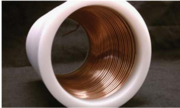
Figure 3: Ferroelectric plasma source (FEPS) that was used in the experiment. The grounded inner electrode is a helical stainless steel winding with a 2 mm pitch. The diameter of the winding is slightly larger than the inner diameter of the  $\text{BaTiO}_3$  cylinder, ensuring good contact between the inner electrode and the ceramic. The ceramic cylinder is enclosed in a Delrin jacket to prevent electrical breakdown.
