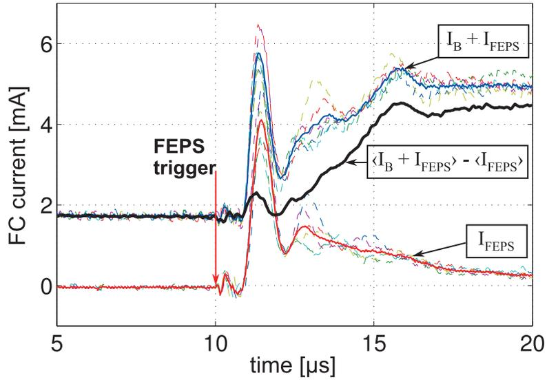
Figure 6: Typical collimated Faraday cup current signals: (blue) average of combined ion beam and FEPS currents ( $\langle I_B + I_{FEPS} \rangle$ ); (red) average FEPS-only current ( $\langle I_{FEPS} \rangle$ ); and (black) ion beam current with the FEPS background subtracted ( $\langle I_B + I_{FEPS} \rangle - \langle I_{FEPS} \rangle$ ). Averages of six signals were used because the FEPS current varied somewhat between individual shots (dashed lines).
