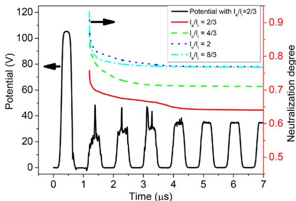
FIG. 4. Temporal evolutions of the potential recorded at  $x = 5$  cm on the axis and the neutralization degrees of the ion beam pulse for different injected electron currents. The size of the computational domain is 40 cm  $\times$  3 cm.
