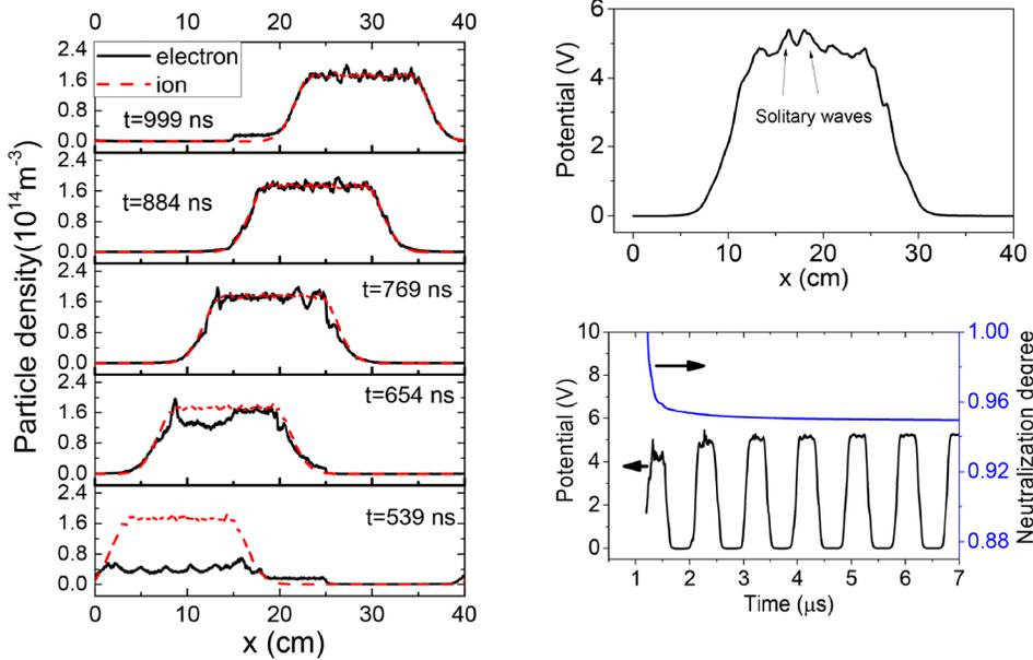
**FIG. 5.** Left: Temporal evolutions of ion and electron densities on the axis. Upper right: Beam potential on the axis at 2.04  $\mu\text{s}$ . Right bottom: Temporal evolutions of the neutralization degree of the ion beam pulse and the potential recorded at  $x = 5$  cm on the axis. Electrons were injected uniformly from  $x = 15$  to 25 cm.
