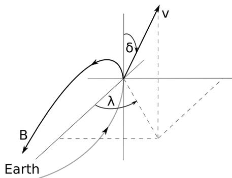
**Figure 1.** Illustration of the angles  $\delta$  and  $\lambda$  which define the orientation of the initial velocity vector of a particle initialized at the midplane of an axisymmetric magnetic field, in this case that of the Earth.
