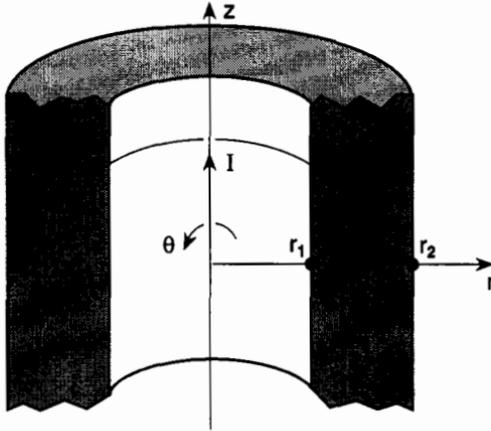
**Figure 19.5.** Annular cylindrical plasma, infinitely long in the  $z$  direction, has a purely azimuthal field  $B_\theta(r)$  produced by the current  $I$  in a central conductor at  $r = 0$ . See Problem 19.2.
