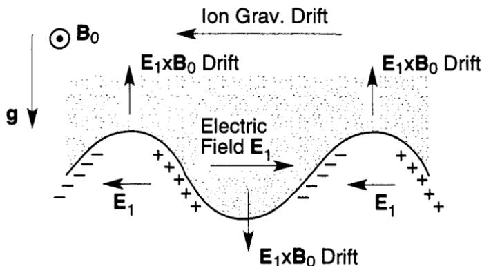
**Figure 19.4.** The mechanism of the Rayleigh–Taylor instability. The ion gravitational drift leads to charge separation on the plasma–vacuum interface, producing electric fields and  $\mathbf{E} \times \mathbf{B}$  drifts that increase the amplitude of the perturbation.
