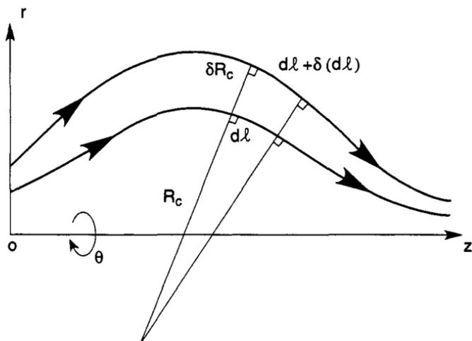
**Figure 19.9.** Two neighboring field lines in a mirror-like configuration with local radii-of-curvature  $R_c$  and  $R_c + \delta R_c$ . The configuration is axisymmetric, i.e. symmetric to rotation in  $\theta$  about the  $z$  axis.
