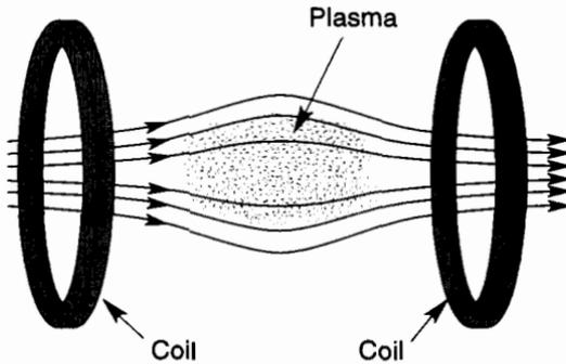
**Figure 19.6.** Plasma equilibrium in a ‘magnetic mirror’ configuration. Note that the magnetic field curvature is concave toward the plasma in the central region where the plasma pressure is largest.
