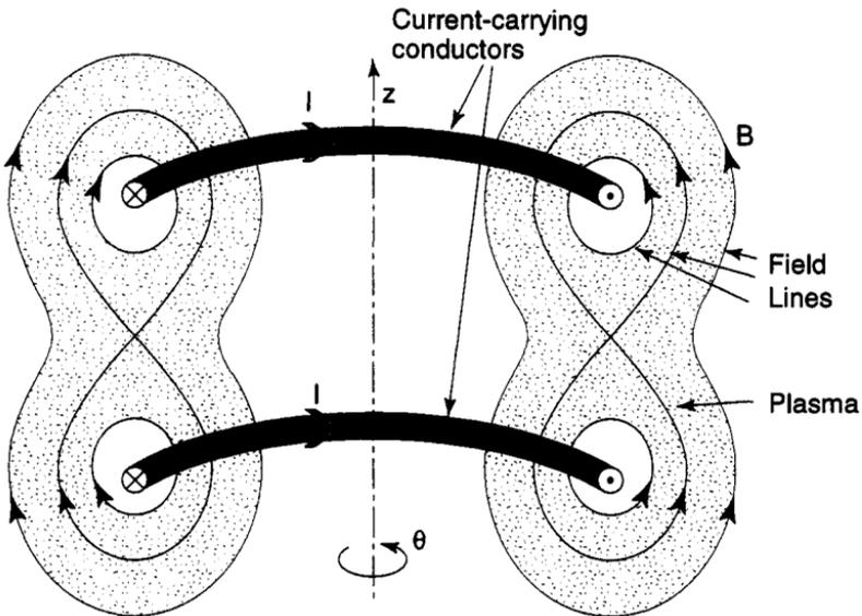
**Figure 19.8.** The toroidal quadrupole configuration. The plasma entirely surrounds the two current-carrying conductors that produce the magnetic field shown. The configuration is axisymmetric, i.e. symmetric to rotation in  $\theta$  about the  $z$  axis.
