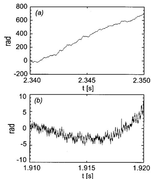
FIG. 10. Time evolution of the signal phase during out-of-focus (a) and in-focus (b) cutoff positions.
