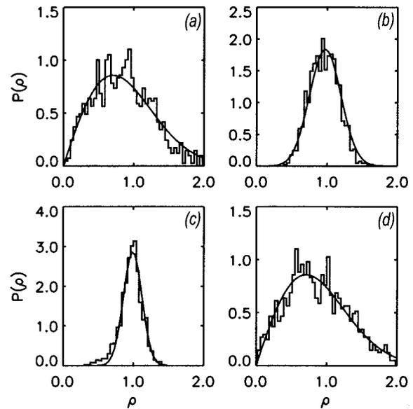
FIG. 9. Amplitude histograms of the signals of Fig. 9 and best fit to a Rice distribution (smooth lines). The Rice parameters  $[\rho_0, \sigma]$  are  $[0.00, 0.71]$  (a),  $[0.95, 0.22]$  (b),  $[0.98, 0.14]$  (c), and  $[0.00, 0.71]$  (d).
