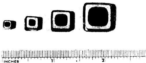
Figure 1: Solid mineral-insulated cables.
