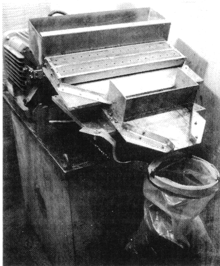
Fig. 26 Magnetic sieve mounted on a vibrator platform
