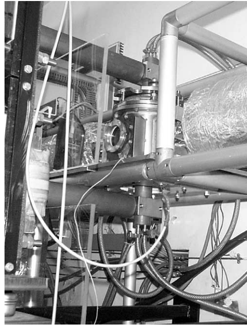
Fig. 3. Thermal hydraulic test rig—heat flux test section.
