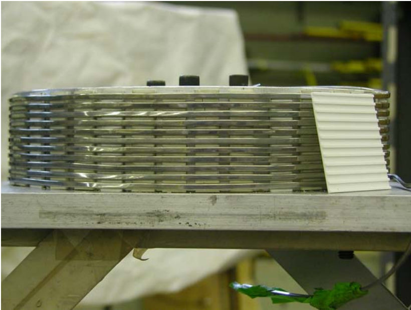
Fig. 3. Cryostable test coil made with alumina insulation. Sample alumina piece is at the right.
