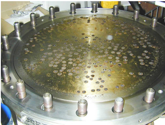
Fig. 2. High vacuum flange after baking cable contaminated with stearic acid ( C_{18}H_{36}O_2 ).
