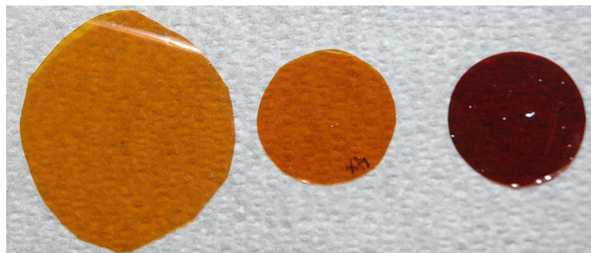
Figure 10. Kapton dielectric specimens. From left to right are examples of the control, 5 \times 10^{22} n/m 2 irradiation, and 5 \times 10^{23} n/m 2 irradiation specimens.
