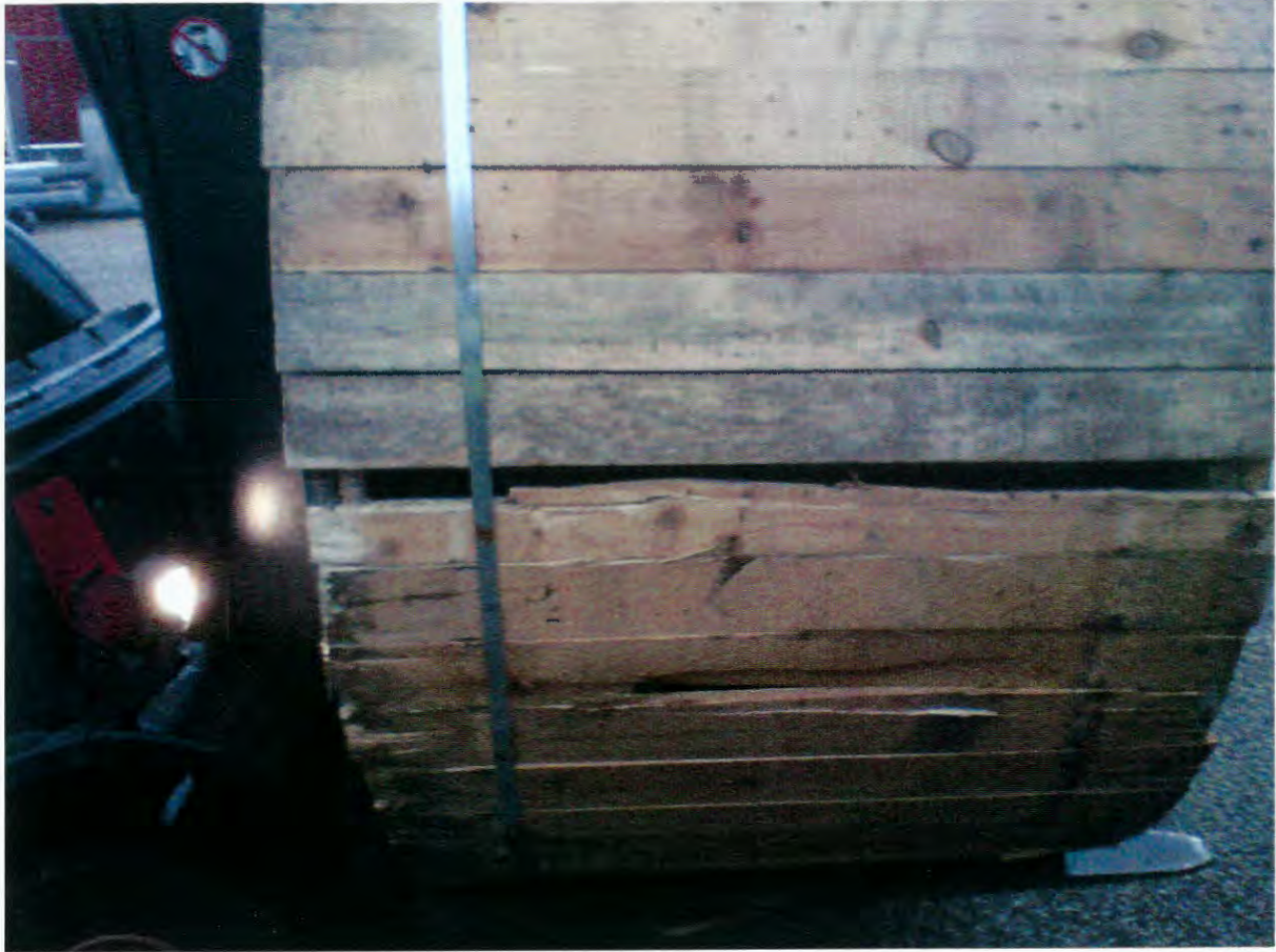
The wooden panels on the cable drum was broken.
