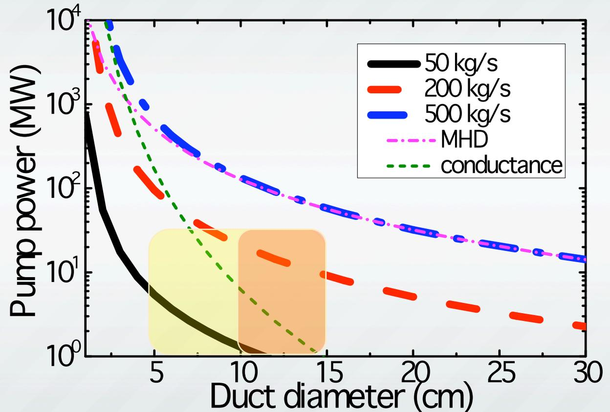
$$\text{Pressure drop} = \text{MHD} + \text{conductance drop}$$
