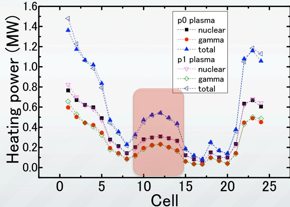
Neutronics result tells how much fraction of nuclear power will be derived to in-board BLKs.
