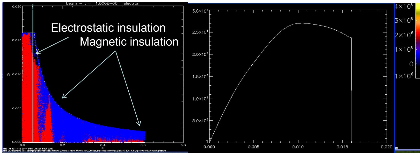
40 MA at 4 MeV injected and 33 MA at 2 MV at load
