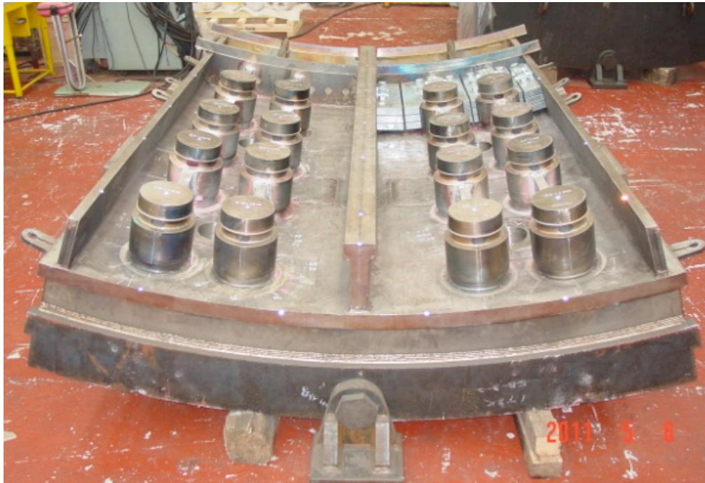
Inboard segment of a VV sector
