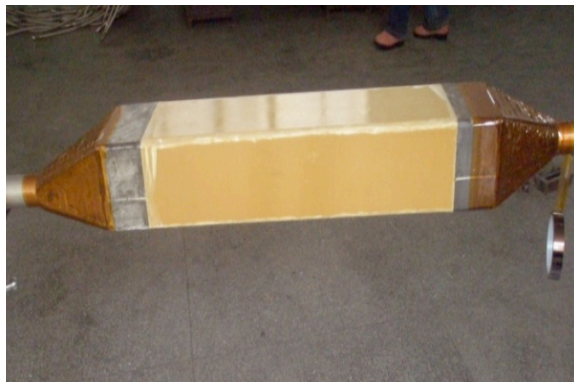
Mid-Joint for Feeder Busbar
