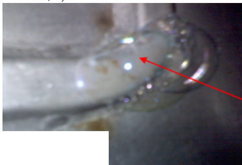
Leaks on the surfaces of the backing channels ( 8.0 \times 10^{-5} mbar l/s).
