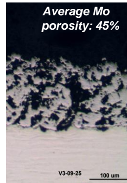
LLD surface cross section: plasma sprayed porous Mo
