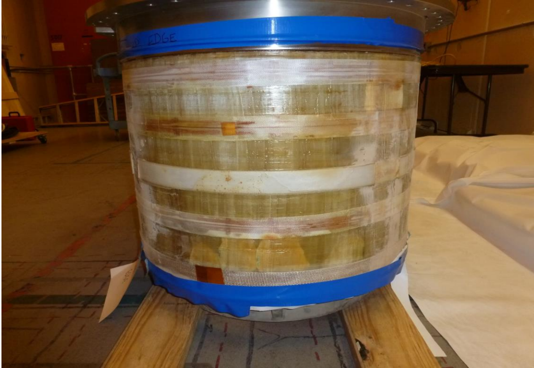
Figure 18 – PF1A-U Exterior with shields removed
