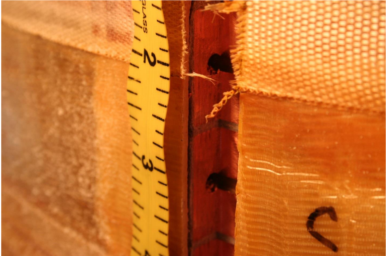
Figure 69 – Cutting Plane C ground wrap delamination
