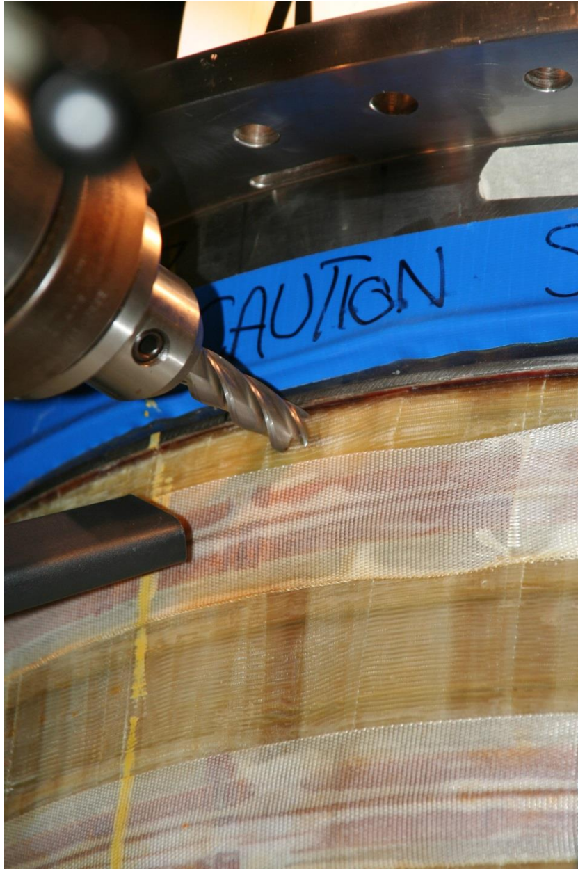
Figure 43 – Four flute end-mill typical of bit used to cut each segment
