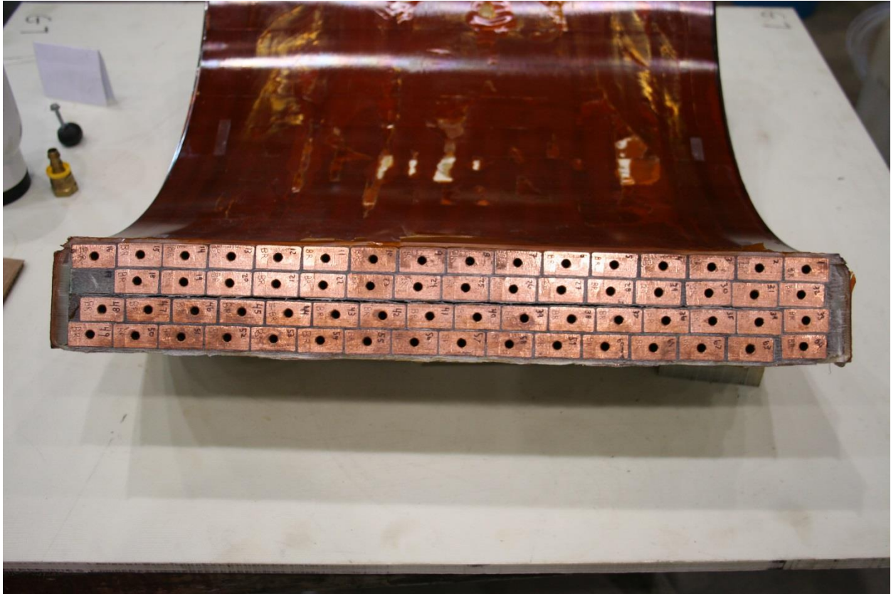
Figure 88 – Coil pack section plane B separation
