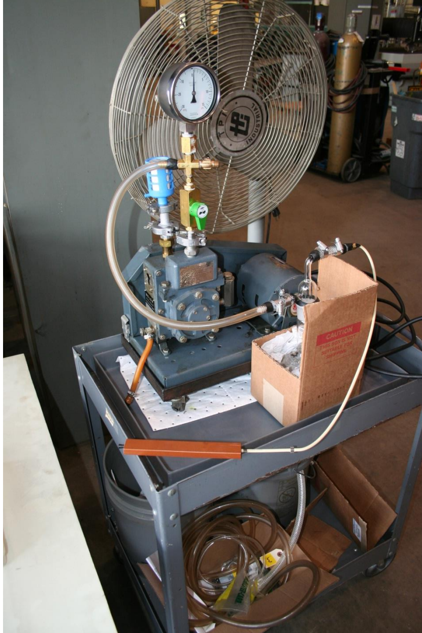
Figure 115 – Vacuum testing apparatus
