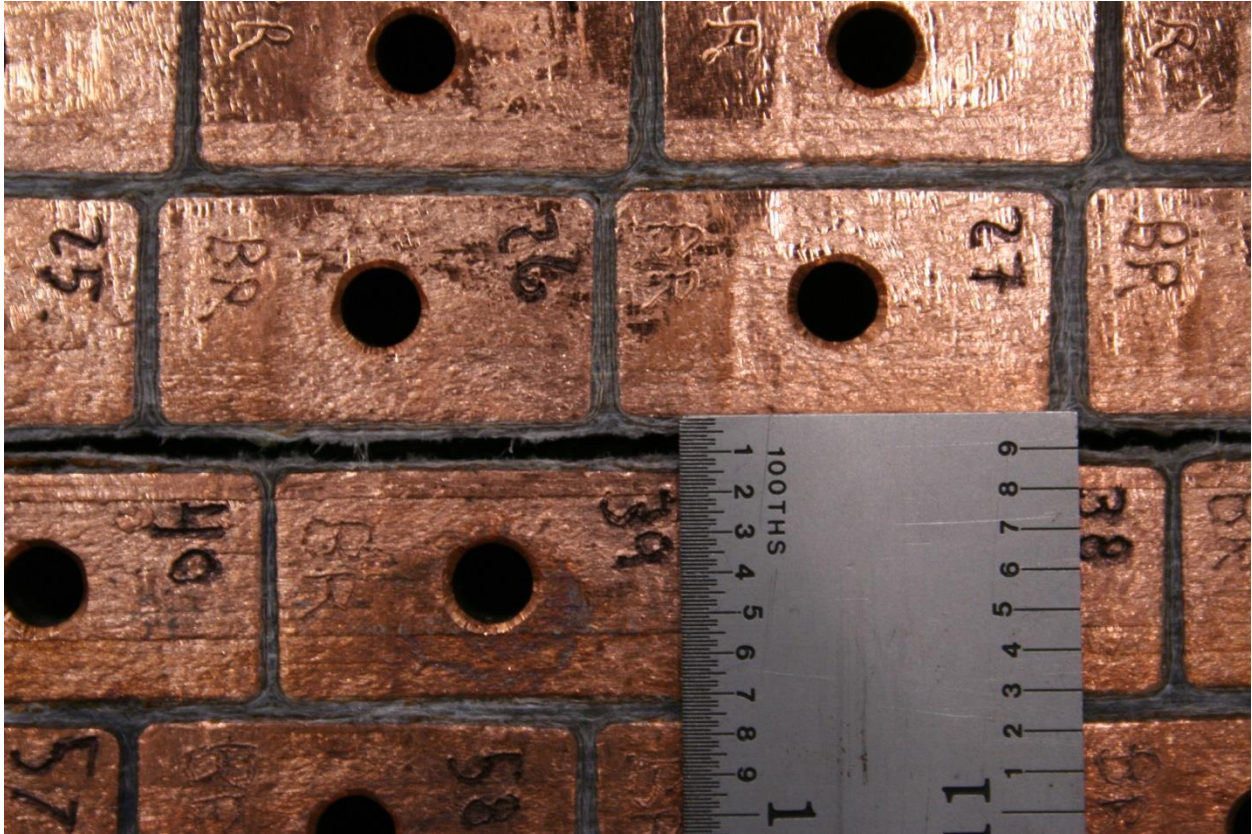
Figure 89 – Coil pack section plane B separation
