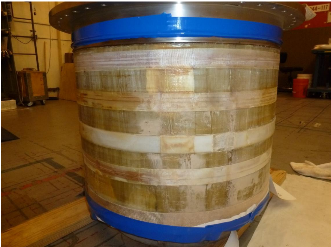
Figure 19 – PF1A-U Exterior with shields removed
