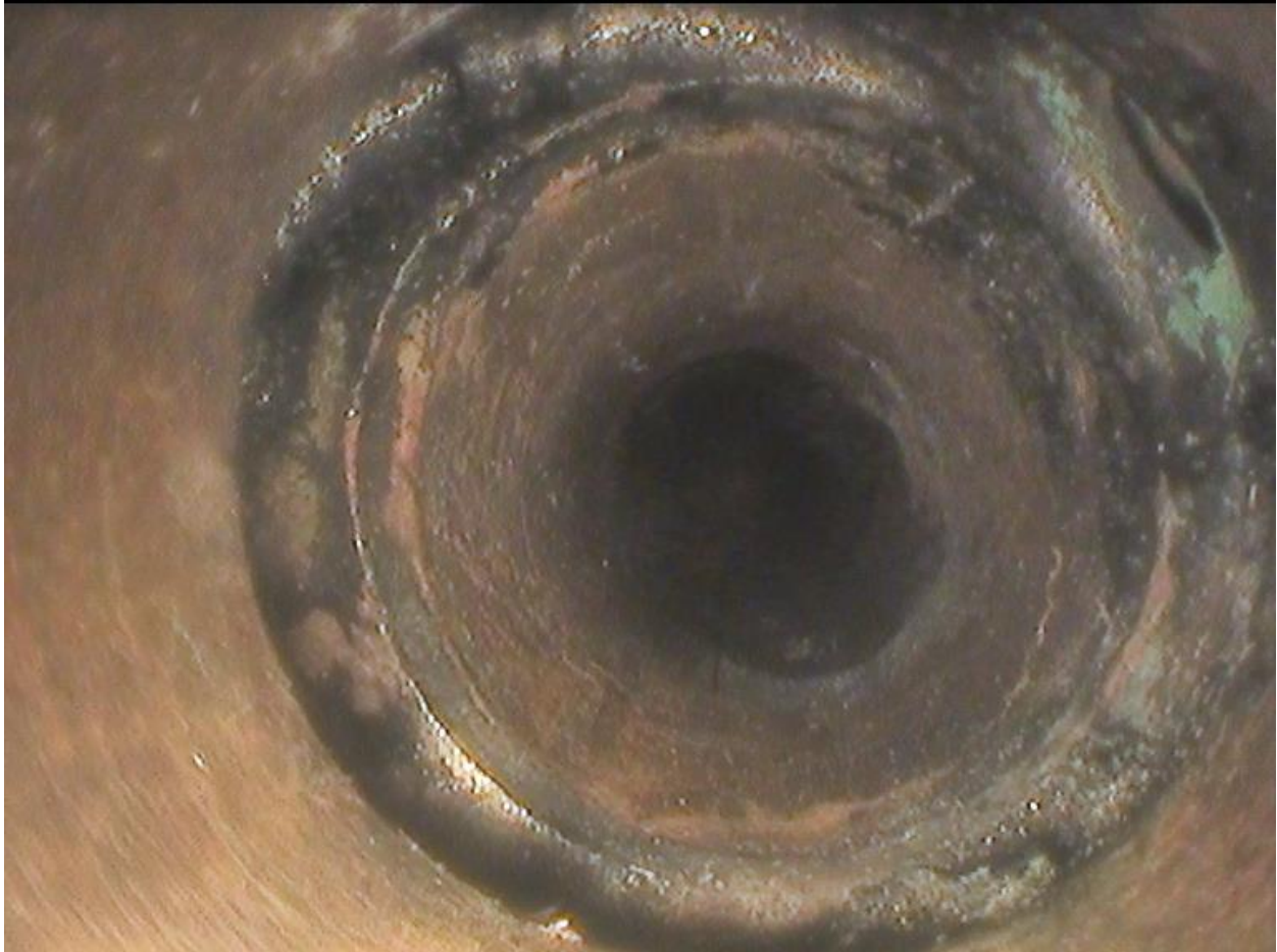
Figure 101 – Braze Joint #2 void – view from plane B
