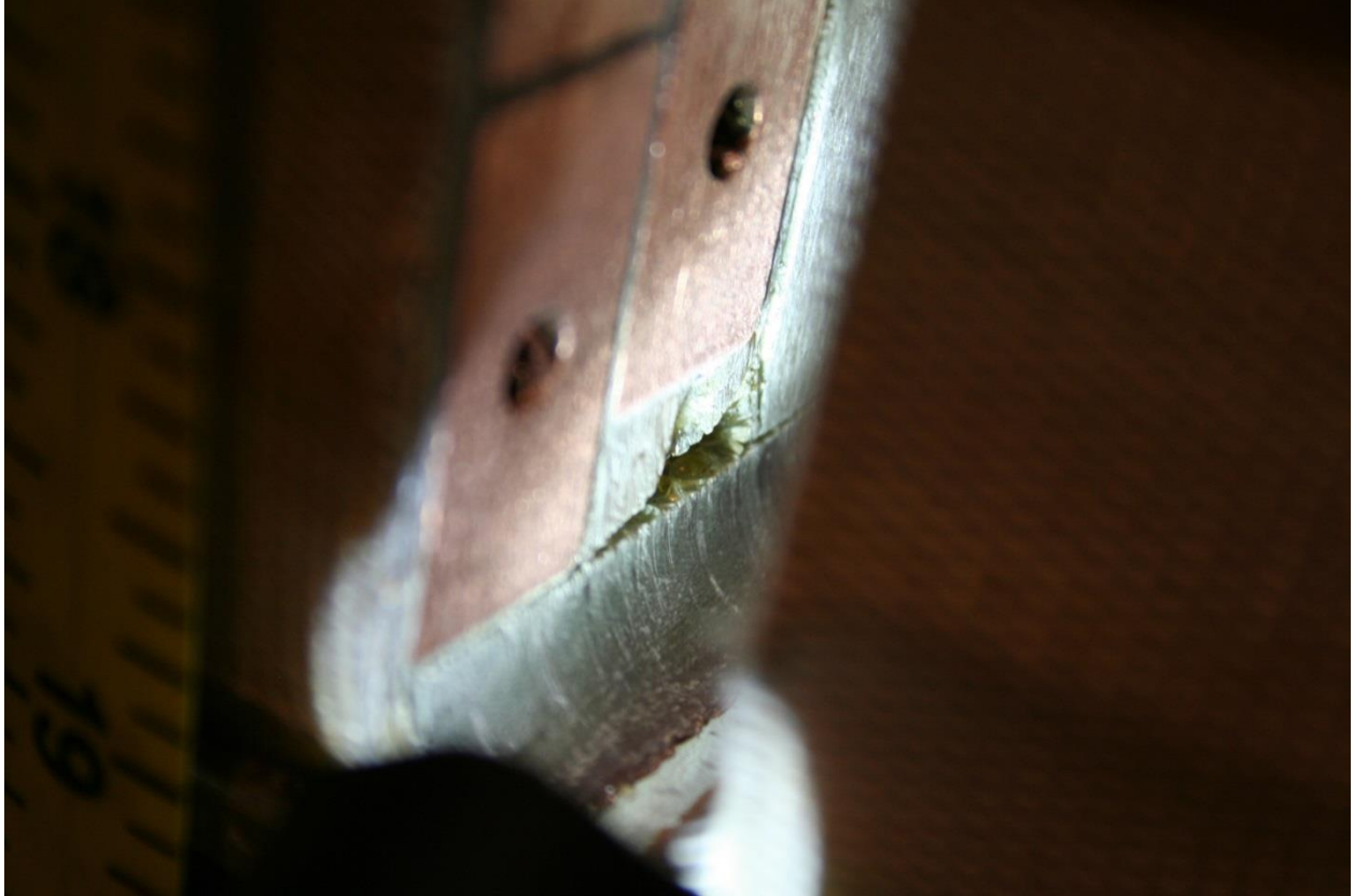
Figure 64 – Cutting Plane B void
