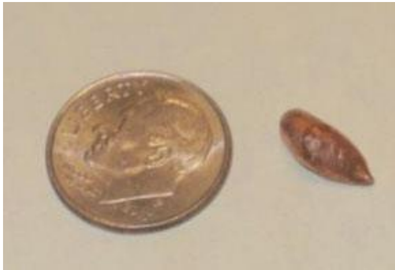
Figure 4 – Copper/carbon slug found in flushed PF1A-U coolant compared to the size of a dime
