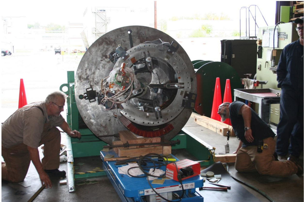
Figure 80 – Coil pack section B_C removal
