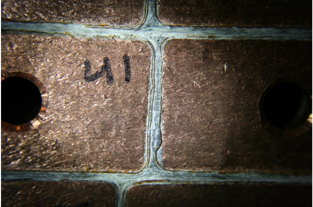
Figure 85 – Coil pack section plane C dry glass
