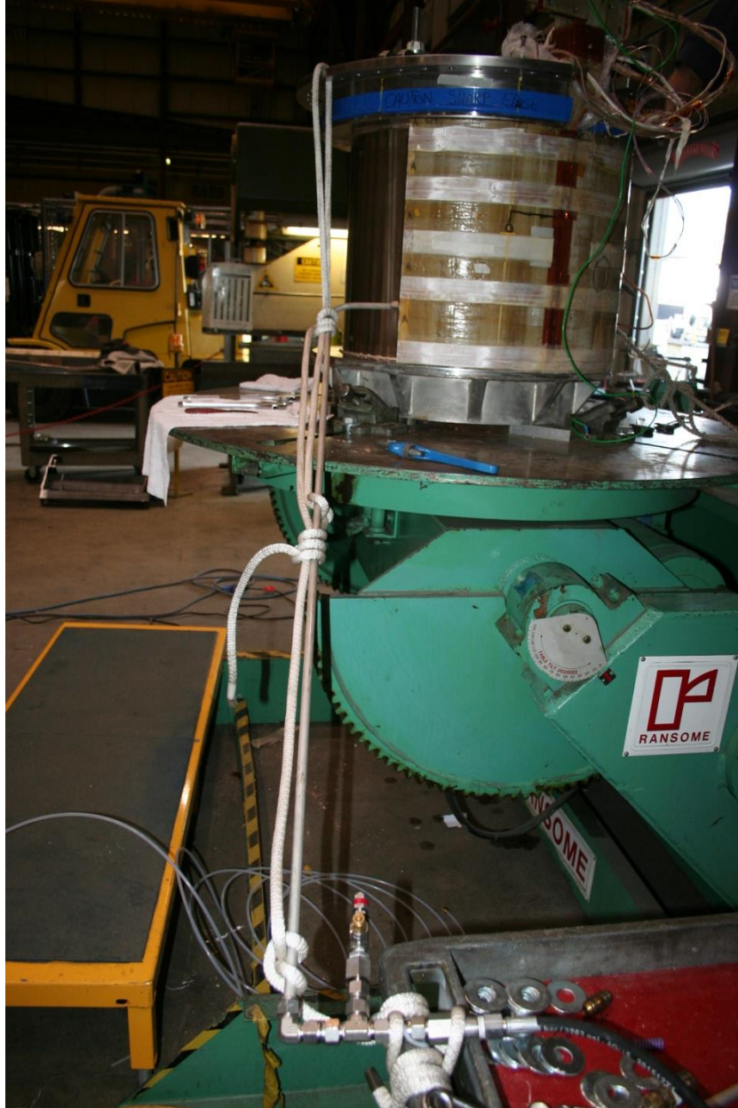
Figure 116 – Pressure testing set-up example
