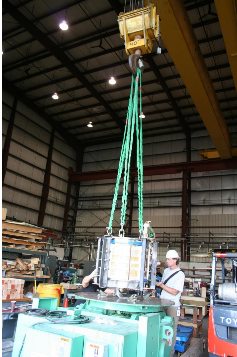
Figure 74 – PF1A-U Placement on Ransome table
