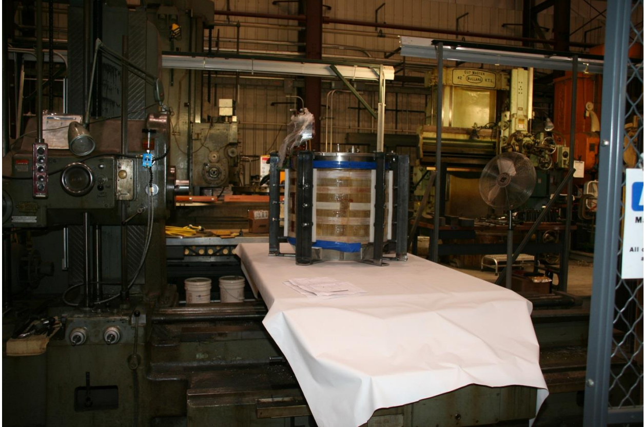
Figure 41 – PF1A-U placement on horizontal Lucas Mill with fixtures
