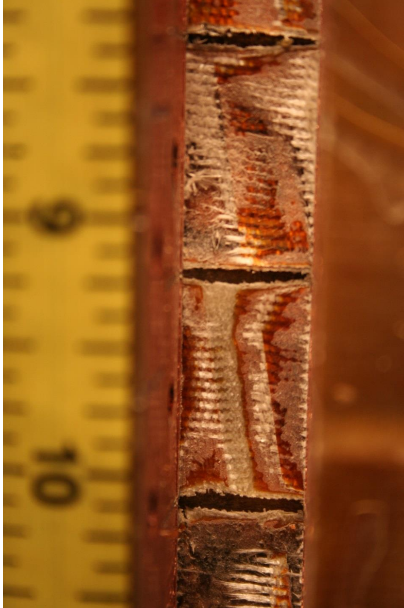
Figure 54 – Cutting Plane B delaminated region
