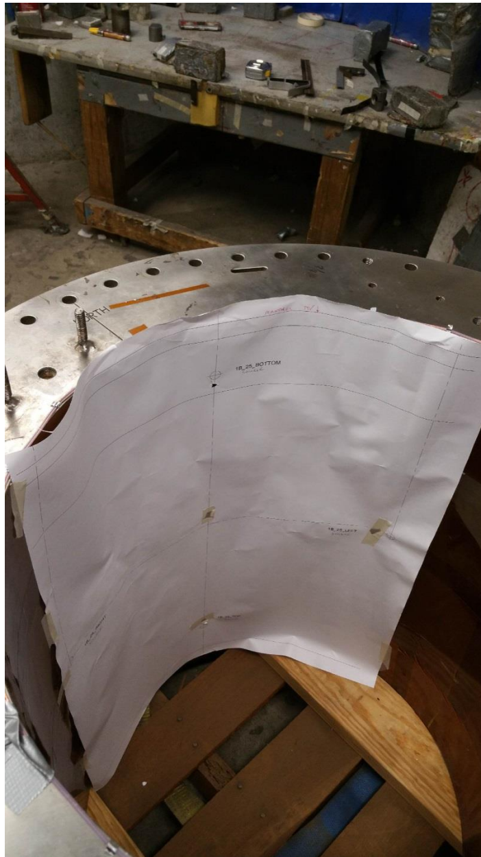
Figure 32 – Inner radius triangulation template for anomalous region 0_1A
