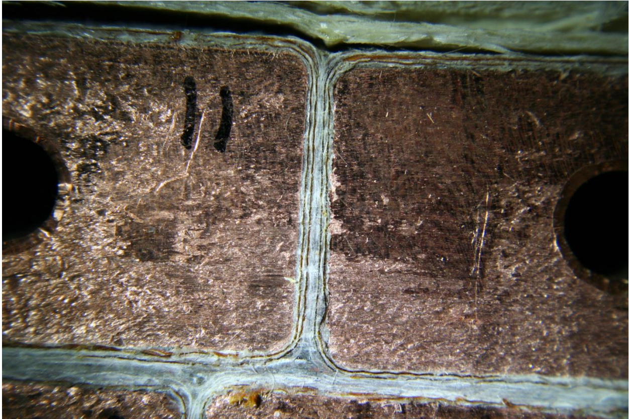
Figure 94 – Coil pack section plane C insulation lay-up
