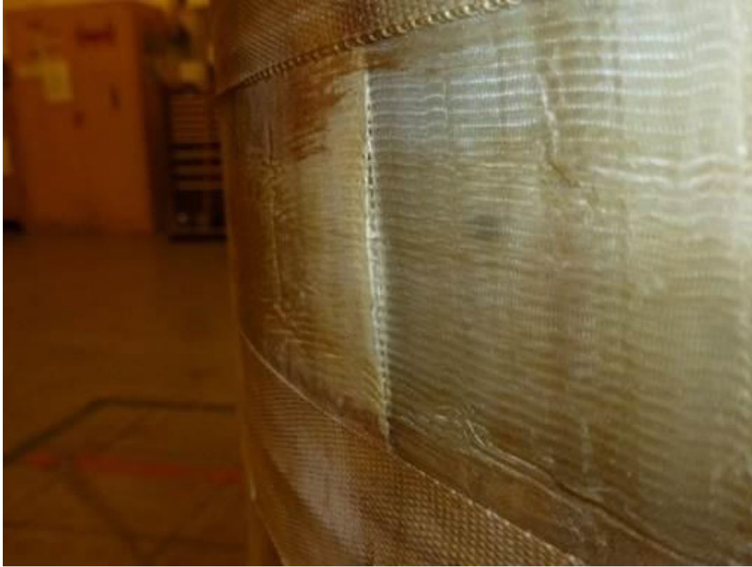
Figure 24 – PF1A-U ground wrap delamination
