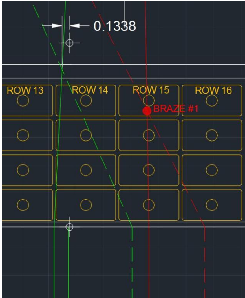
Figure 39 – AutoCAD-based triangulation of Braze Joint #1
