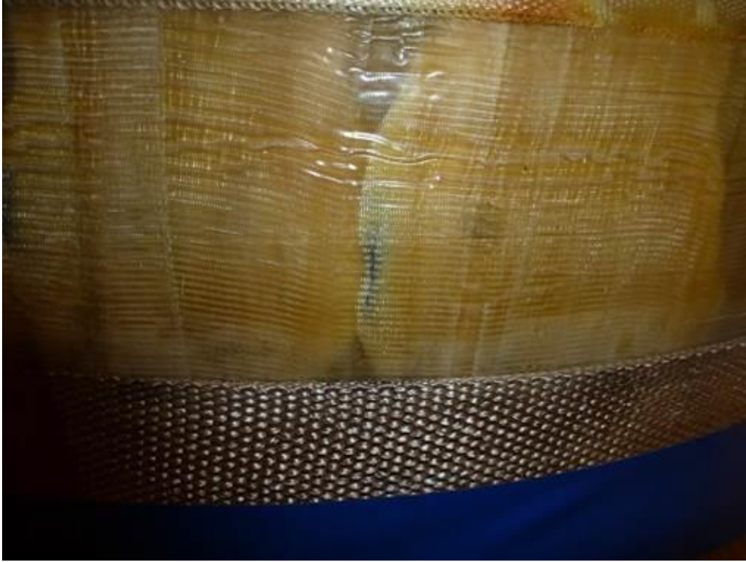
Figure 20 – PF1A-U ground wrap delamination
