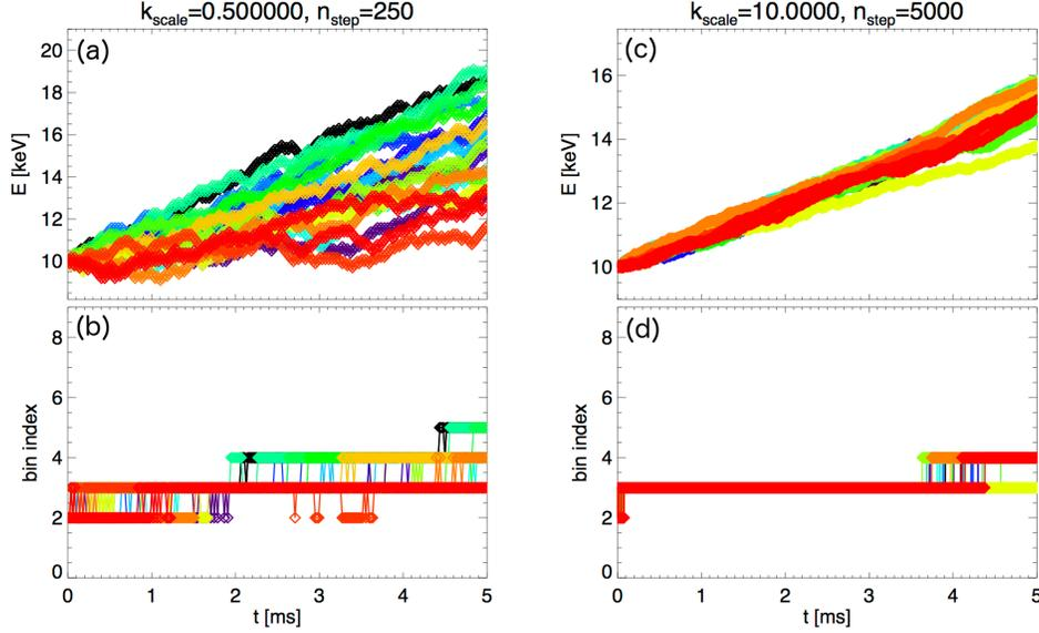
FIG. 1. Test of MonteCarlo particle (a,c) energy trajectories and (b,d) bin index vs. time. Each color represents a different MonteCarlo run for particles with the same initial energy,  $E_0 = 10$  keV. The number of MonteCarlo steps to cover the 5 ms interval is increased from 250 to 5000 from (a,b) to (c,d).
