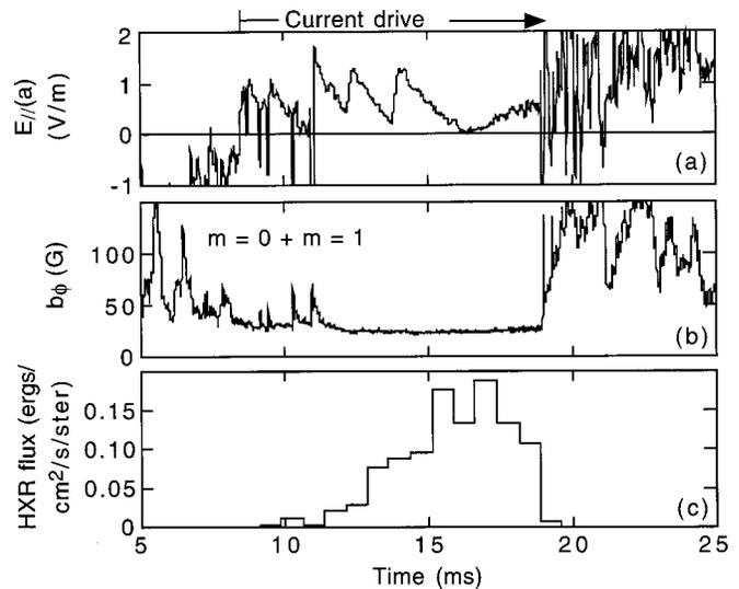
FIG. 5. From a 500 kA plasma with auxiliary current drive (a) surface parallel electric field, (b) rms sum of  $m=0$  and  $m=1$  toroidal magnetic fluctuations with  $n=1-15$ , and (c) hard-x-ray flux.
