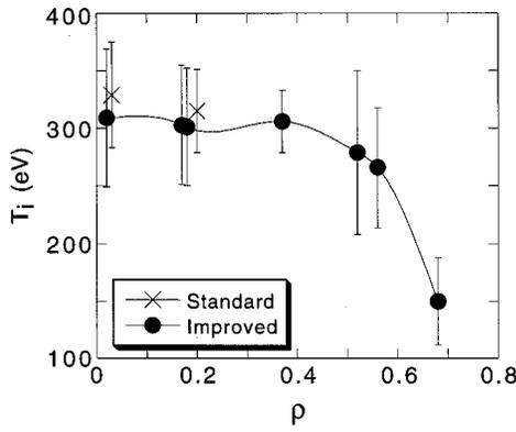
FIG. 9.  $C^{+6}$  ion temperature profiles in 500 kA standard- and improved-confinement plasmas.
