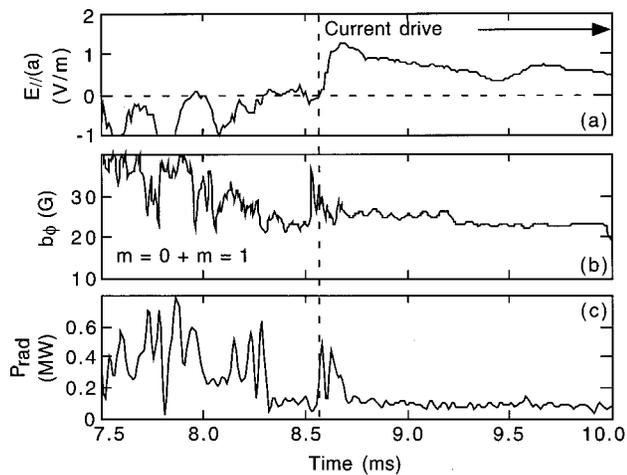
FIG. 4. From the plasma on the right in Fig. 3, (a) surface parallel electric field, (b) root-mean-square (rms) sum of  $m=0$  and  $m=1$  toroidal magnetic fluctuations with  $n=1-15$ , and (c) total radiated power (photons only).
