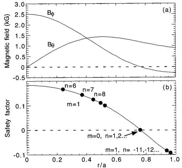
FIG. 2. Estimated profiles of (a) toroidal and poloidal magnetic fields, and (b) the safety factor for a 230 kA plasma with strong toroidal magnetic field reversal. Locations of  $m=1$  and  $m=0$  resonant surfaces are indicated.
