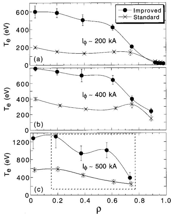
FIG. 7. Electron temperature profiles from standard- and improved-confinement plasmas at three plasma currents with a central line-averaged density of (a)  $\sim 8 \times 10^{18} \text{ m}^{-3}$ , (b)  $1 \times 10^{19} \text{ m}^{-3}$ , and (c)  $9 \times 10^{18} \text{ m}^{-3}$ . The central temperatures at 500 kA are averages over more than ten shots, but the other 500 kA data points (within the dashed box) are averages over less than five shots.
