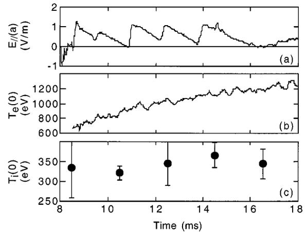
FIG. 8. (a) Surface parallel electric field and (b) central electron temperature from the 500 kA plasma on the right in Fig. 3, and (c) central  $\text{C}^{+6}$  ion temperature compiled from many similar 500 kA shots.
