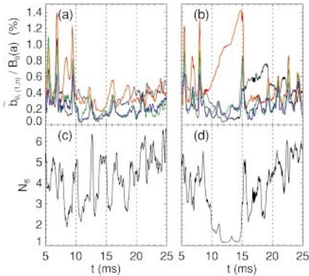
FIG. 1. (Color) Time evolution of the magnetic  $m = 1$  modes measured with a toroidal array of magnetic field sensing coils at the plasma surface. Amplitudes of  $m = 1$ ,  $n = 5 - 8$  and the spectral spread  $N_s$  for a MH plasma (a), (c) and for a spontaneous QSH plasma (b), (d) are shown (black:  $n = 5$ ; red:  $n = 6$ ; green:  $n = 7$ ; blue:  $n = 8$ ).
