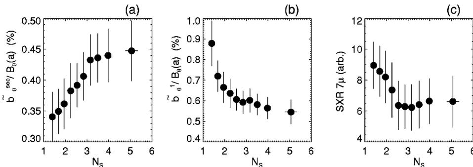
FIG. 3. (a) Normalized rms secondary modes,  $b_\theta^{\text{sec}}/B_\theta(a)$  vs  $N_s$ . (b) Normalized rms of all  $m = 1$  modes,  $\sqrt{\sum b_\theta^2}/B_\theta(a)$ , vs  $N_s$ . (c) SXR emission measured through a  $7 \mu\text{m}$  thick beryllium filter vs  $N_s$ .
