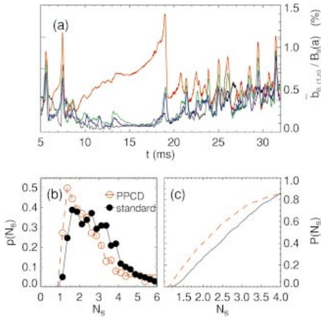
FIG. 4. (Color) (a) Time evolution of the magnetic  $m=1$  mode amplitudes during a PPCD shot where a QSH spectrum appears. (b) Probability density distributions of  $N_s$  for plasmas with and without PPCD. (c) Probability curve of obtaining a given value of  $N_s$  for PPCD and standard plasmas.
