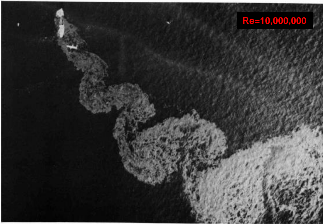
173. Wake of a grounded tankship. The tanker Argo Merchant went aground on the Nantucket shoals in 1976. Leaking crude oil shows that she happened to be inclined at about 45^\circ to the current. Although the Reynolds
